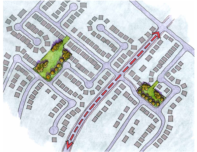
Illustration 5. This neighbourhood includes two neighbourhood parks. Residents on each side of the arterial road have access to a park without the need to cross the arterial.
