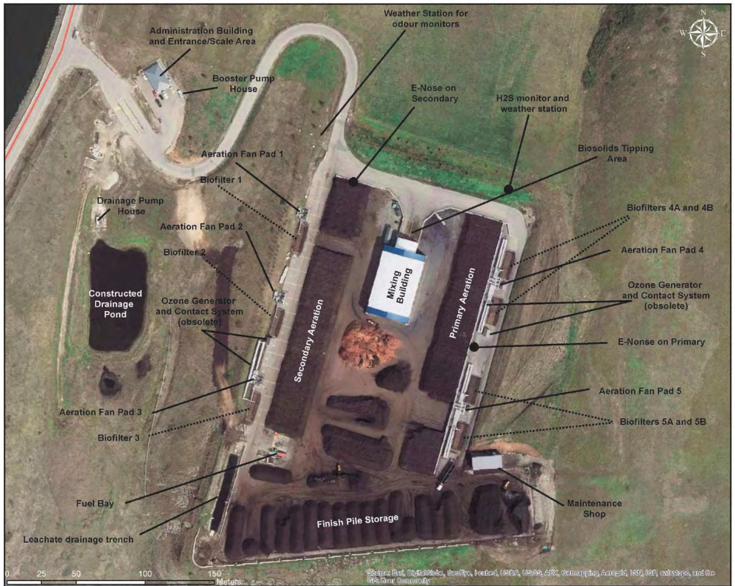
Figure 1. Regional Compost Facility Site Plan
