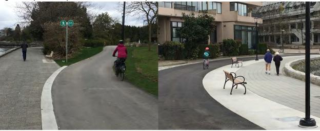
Separated bicycle pathways can be designed to accommodate either uni-directional or bi-directional bicycle travel. Separated pedestrian pathways should be designed to be bi-directional and allow people to travel side-by-side and to accommodate users travelling in the opposite directions. General guidance on widths is provided in the table below.
